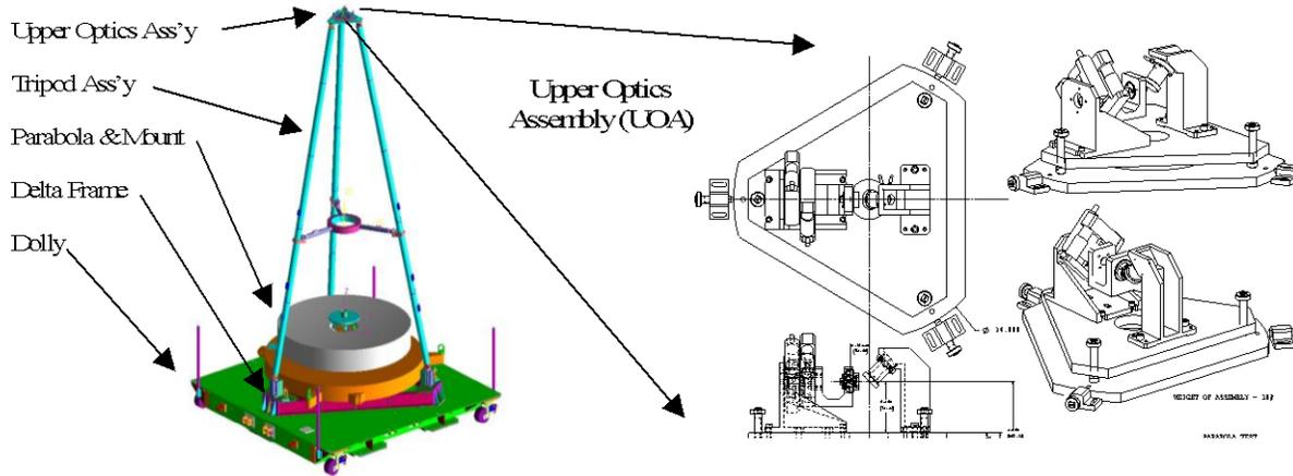
Fig. 3. Parabola Test Assembly with Details of the Upper Optics Assembly.
