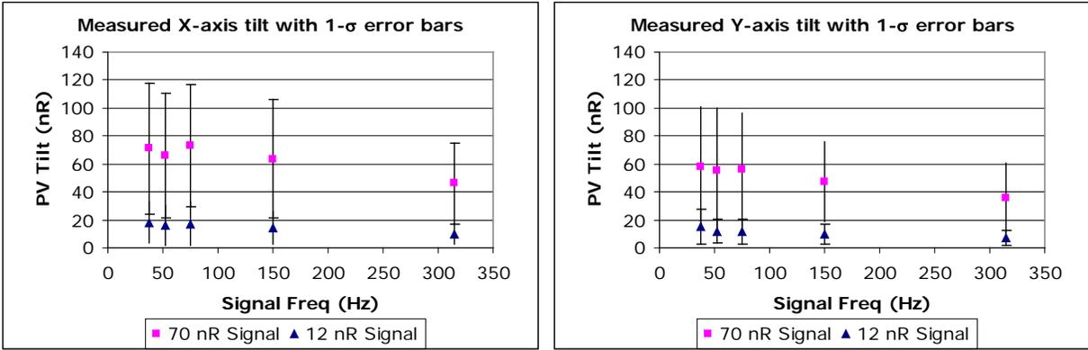
Fig. 13. Signal amplitudes with 1- $\sigma$  error bars ( $\pm$  standard deviation). There is a trend downward in measured signal strength with increasing frequency for both directions and test amplitudes. This indicates the PZT travels less distance during high-frequency oscillations. Improved calibration would compensate for this behavior. The large error bars show the large variation in individual sensor measurements, though the mean detected signal is close to the actual input signal.
