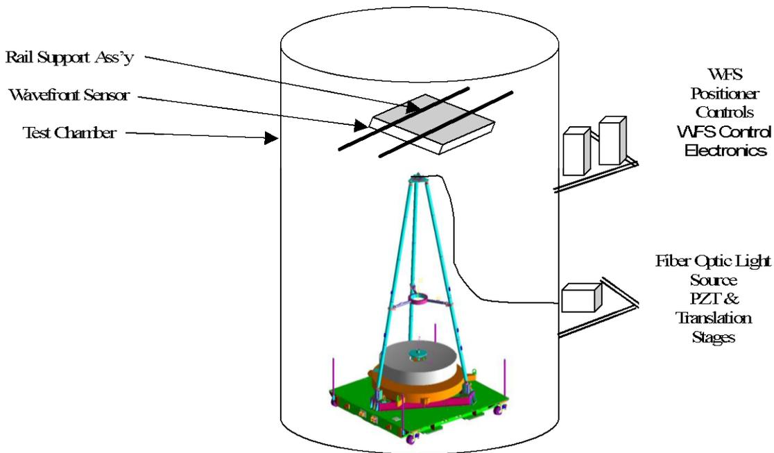
Fig. 4. WFS test assembly inside chamber, below the Wavefront Sensor.
