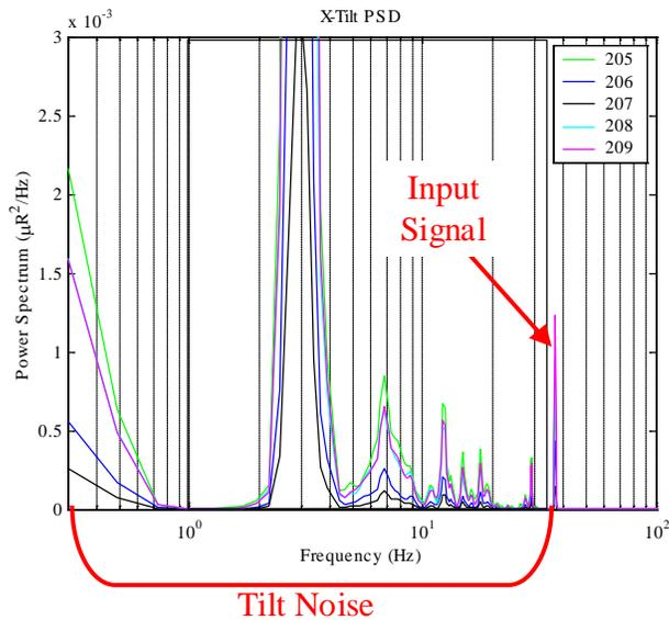
Fig. 11. Typical PSD curves from wavefront tilt data. Here the input signal was at 37 Hz and was the only optical signal. But environmental noise vibrated the WFS test equipment, causing mechanical tilts relative to the optical beam which were detected as optical tilts. The noise is primarily below 30 Hz but has significantly more energy than the test signal. Here, the test signal is a 35 nR RMS amplitude sinusoid and the total noise from 1 to 30 Hz is about 200 nR RMS.
