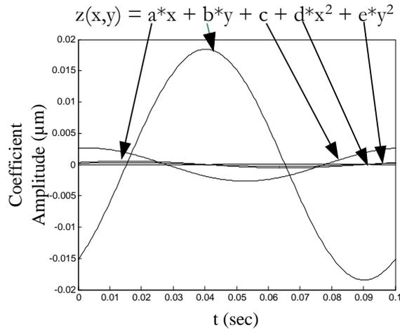
Fig. 8. Dynamic coefficients for one PZT test at 10Hz, equivalent to a 244 nR wavefront tilt. Ideally the  $b$  coefficient would be the only non-zero coefficient, reflecting pure vertical tilt.
