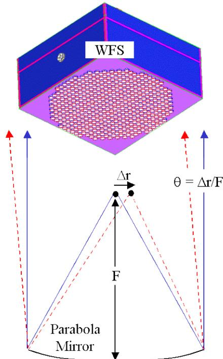
Fig. 1. The WFS test is achieved by moving the light source laterally about the parabola focal point, dynamically titling the collimated output beam. The wavefront slope is proportional to the source motion ( $\Delta r$ ) and the focal length of the mirror ( $F$ ).
