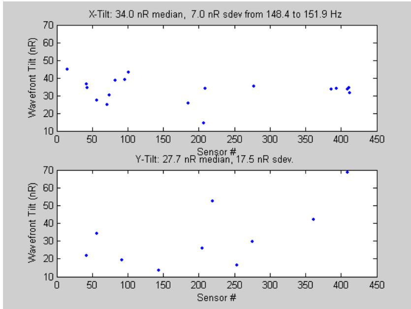
Fig. 14. Analysis of sensors with gain values within  $\pm 1/2\%$  of nominal value. The error is reduced substantially.
