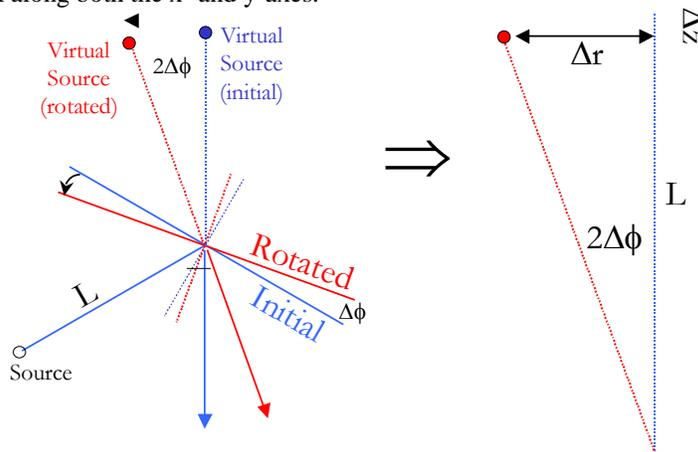
Fig. 2. Tilting a fold mirror causes translation of the virtual source (the reflection of the physical source). For small tilts, the virtual source motion is almost pure translation, relative to the initial reflected beam.
