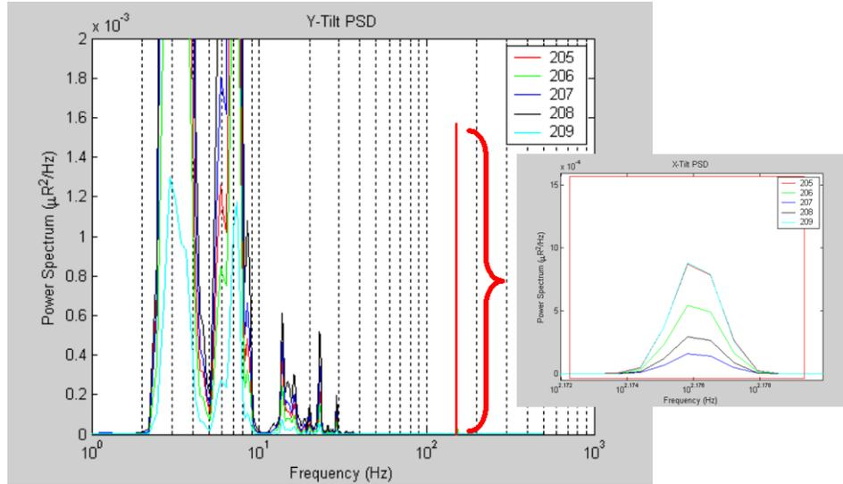
Fig. 12. Y-tilt PSD curve with 150 Hz test signal selected for analysis, highlight in red. The selected region is shown in the inset figure. Sinusoidal input signals have a Gaussian PSD form.
