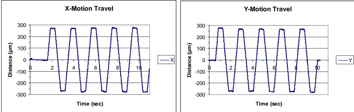
Fig. 6. Measured motion for front stage, for a  $\pm 272 \mu\text{m}$  trapezoidal pattern
