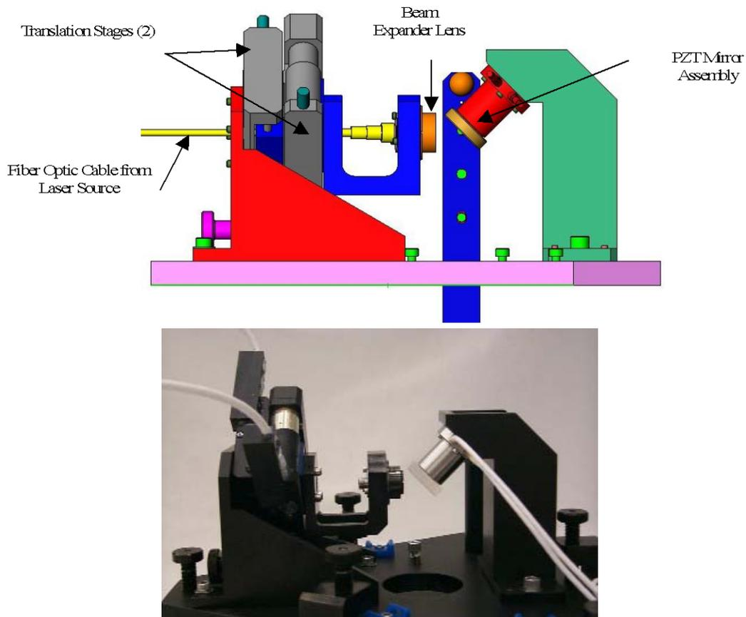
Fig. 5. Schematic of Upper Optics Assembly (top) and photograph of hardware (bottom). The translation stages, on the left, provide  $540 \mu\text{m}$  of linear motion to steer the output beam during WFS calibration. The PZT tilts its attached fold mirror  $10 \mu\text{R}$  to steer the beam for WFS tilt sensing testing.
