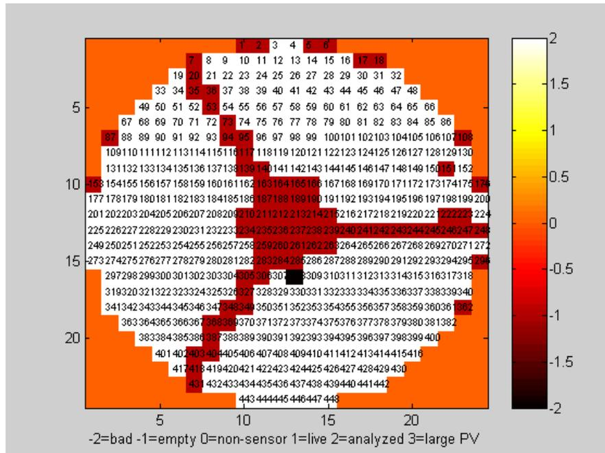
Fig. 10. WFS map with sensor numbers labeled. White are valid, analyzed sensors. Dark red are “empty” sensors reporting zero tilt at all times. Most empty sensors are those obstructed by test-set hardware (tripod & UOA) or are at the edge of illumination, though sensor 151 may be a failed sensor. The black square is a bad sensor and reports invalid tilts. And sensor 308 was dead for tests analyzed.
