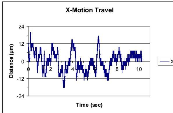
Fig. 7. Crosstalk along x-axis during y-translation measurement.
